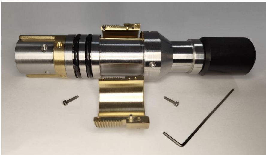
Figure 6-1.2 Ring halves when pulled apart
