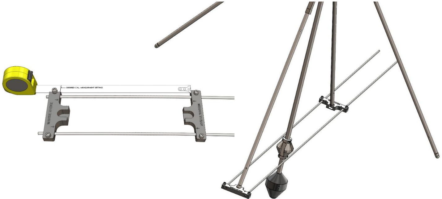
Figure 5-1.1 Using the Field Calibration Kit
