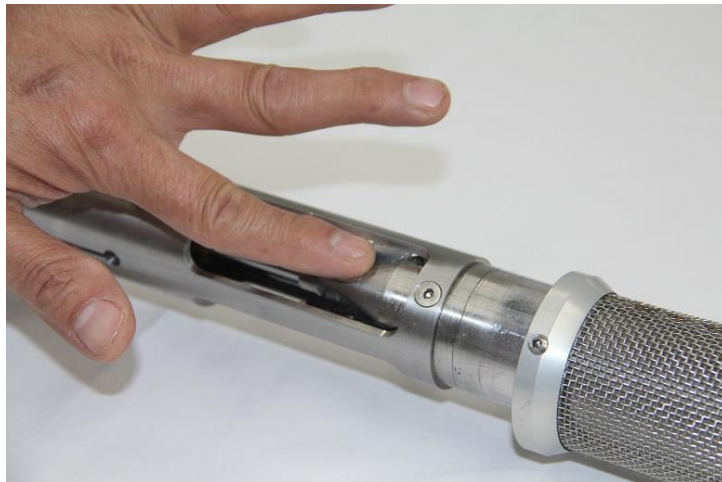
Figure 5-7 Use finger to be sure grease fills all crevasses and gaps.
