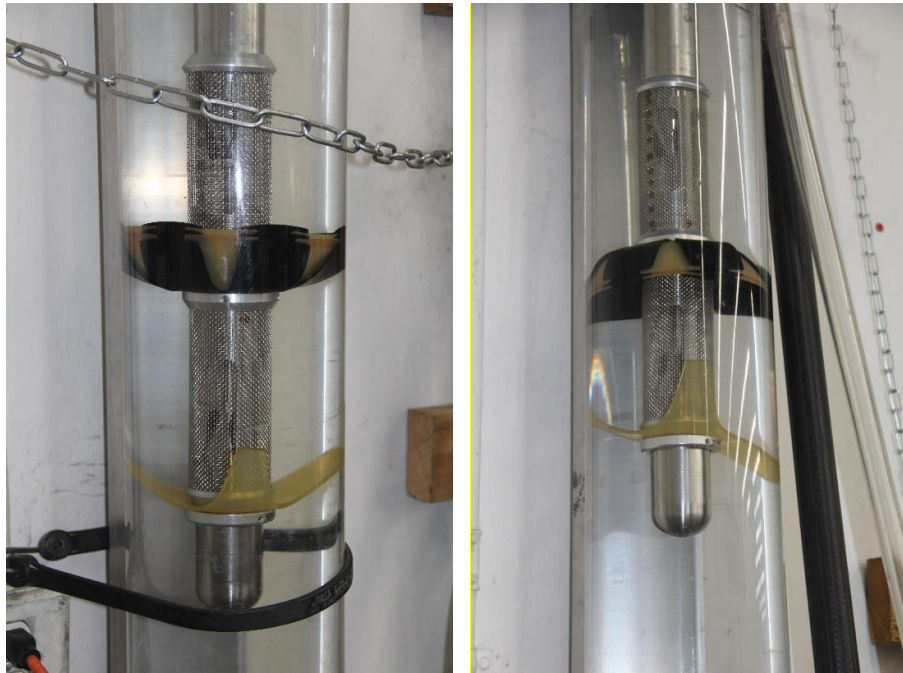
Figure 3-6. Heat-Pulse Flowmeter showing diverter petals in up position for downward flow (left) and down position for upward flow (right).
