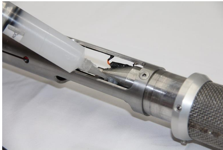
Figure 5-6 Correct application of grease around mecca boot within the bulkhead cut-outs.
