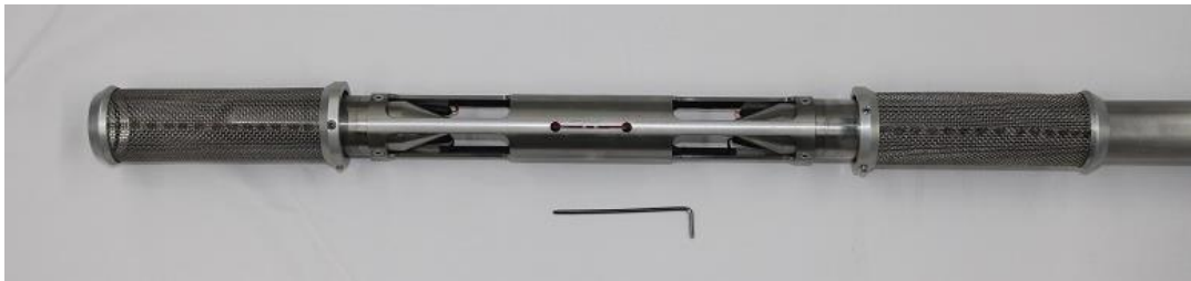
Figure 5-2 Heat pulse with screens removed.
