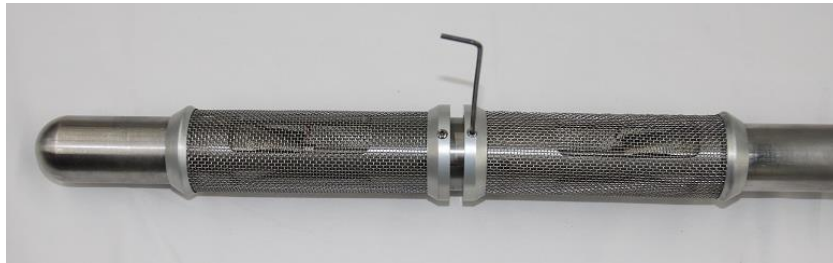
Figure 5-1 Remove the Heat Pulse screens with Allen wrench
