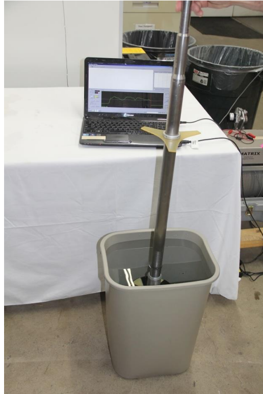
Figure 4-7 Erratic signal shown just after probe enters the water.
