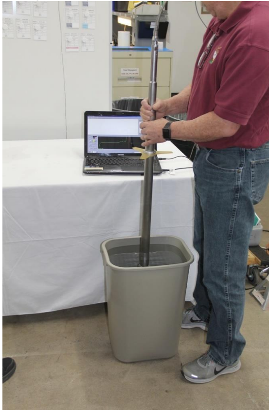
Figure 4-9 Positive peak indicates upward flow after lowering probe.
