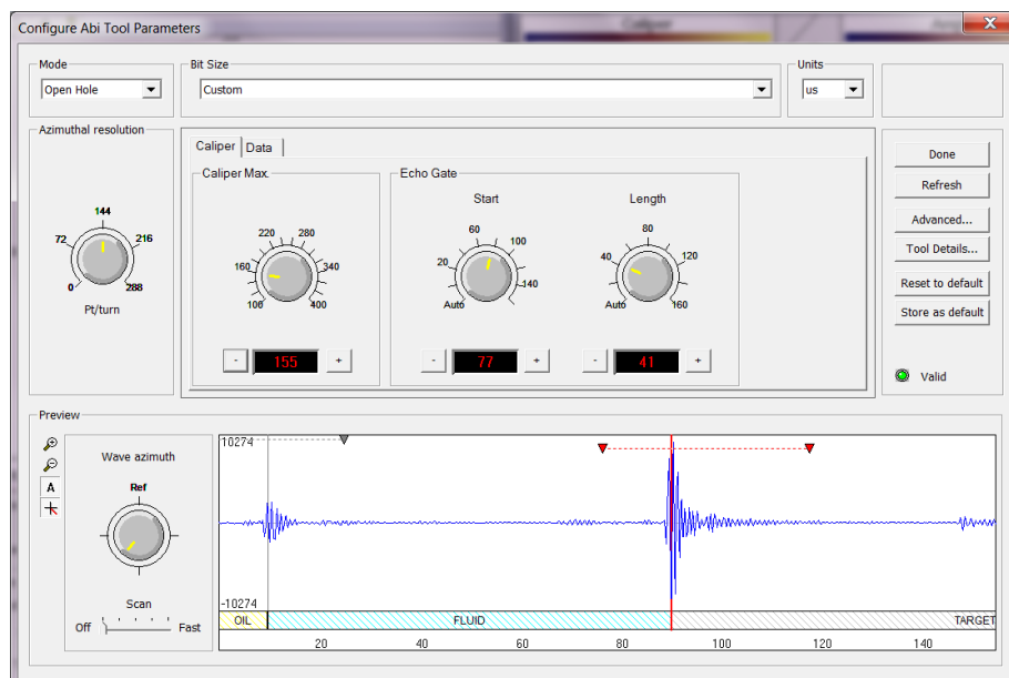
Figure 3-6 Tool settings – Open Hole Mode (caliper scale here in µs)
