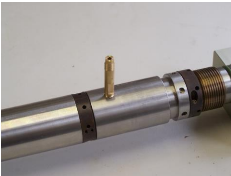
Oil filler screwed in the oil filling hole
