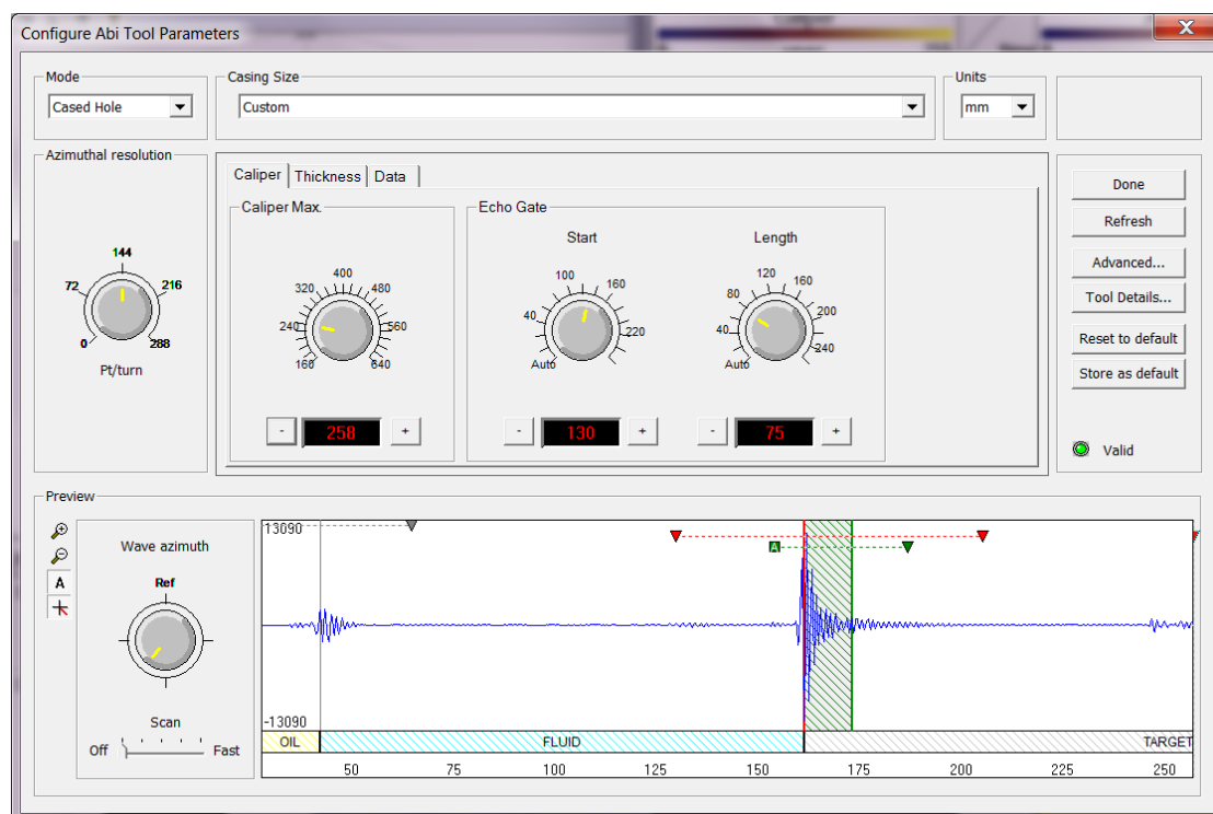
Figure 3-18 Example of Cased hole settings
