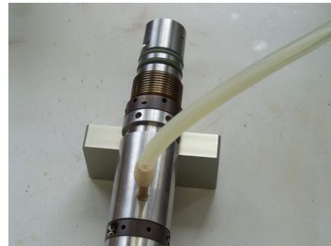
Vacuum pump tube fixed on the oil filler screw
