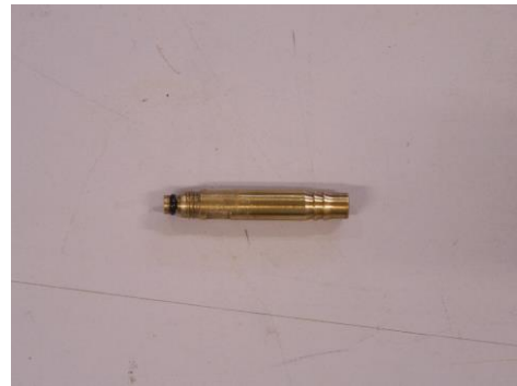
O-Ring set on the oil filler
