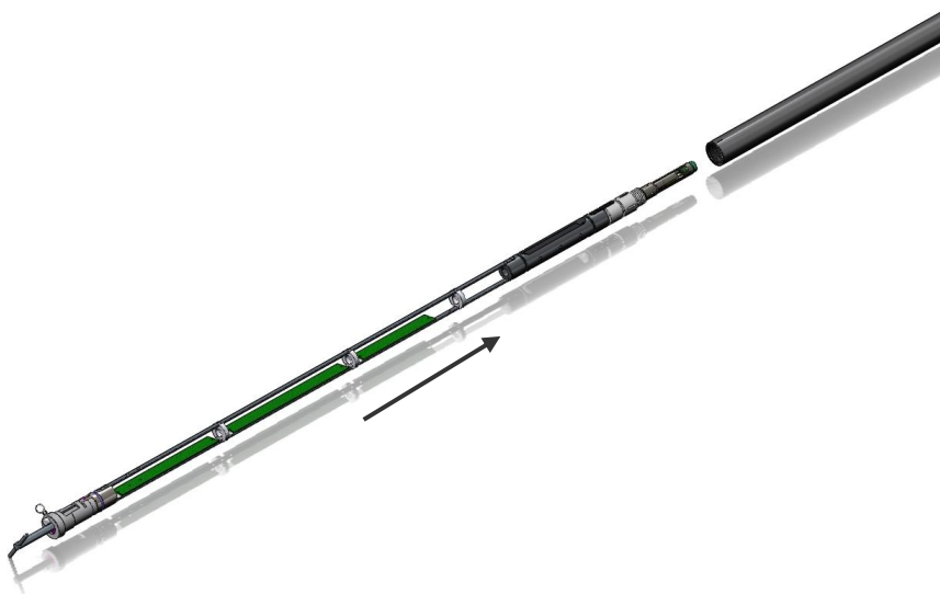
Figure 5-39 Inserting the electronics into the pressure housing
