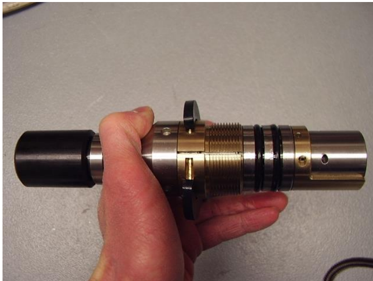
Figure 6-2 Disassembly of the locking ring –step 1
