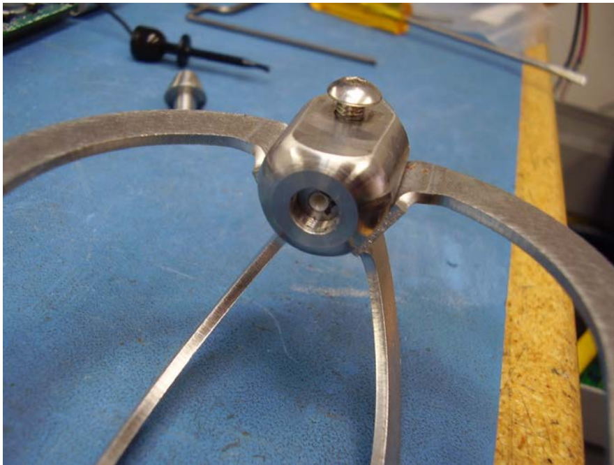
Figure 3-2 Cup detailed picture of the cup for the impeller axle bearing
