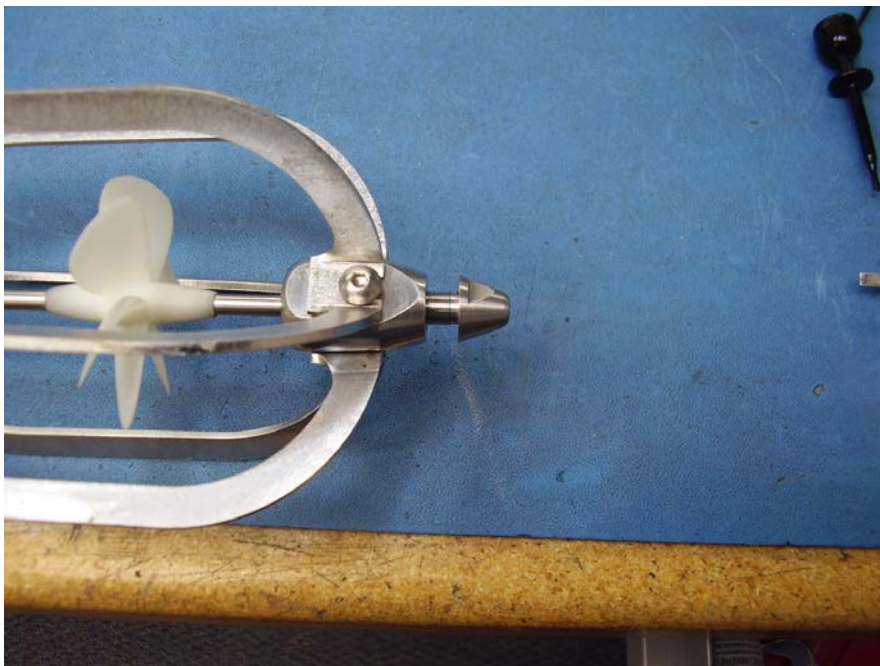
Figure 3-5 Installation of the lower cone and final check
