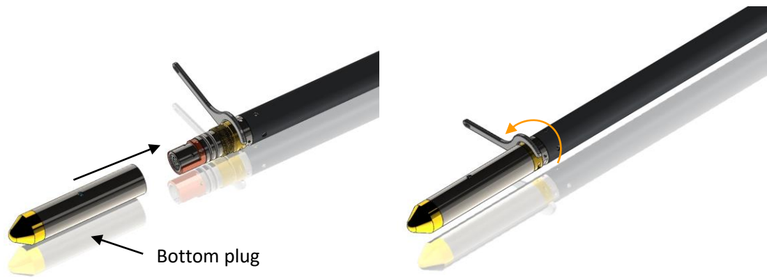
Figure 3-4 Attaching the QL40-Plug
