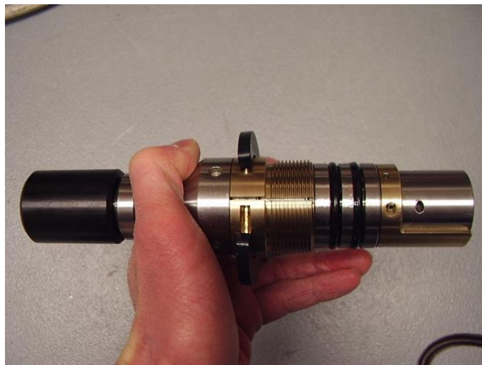
Figure 6-2 Disassembly of the locking ring –step 1
