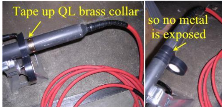
Figure 3-5 bridle connection and isolation
