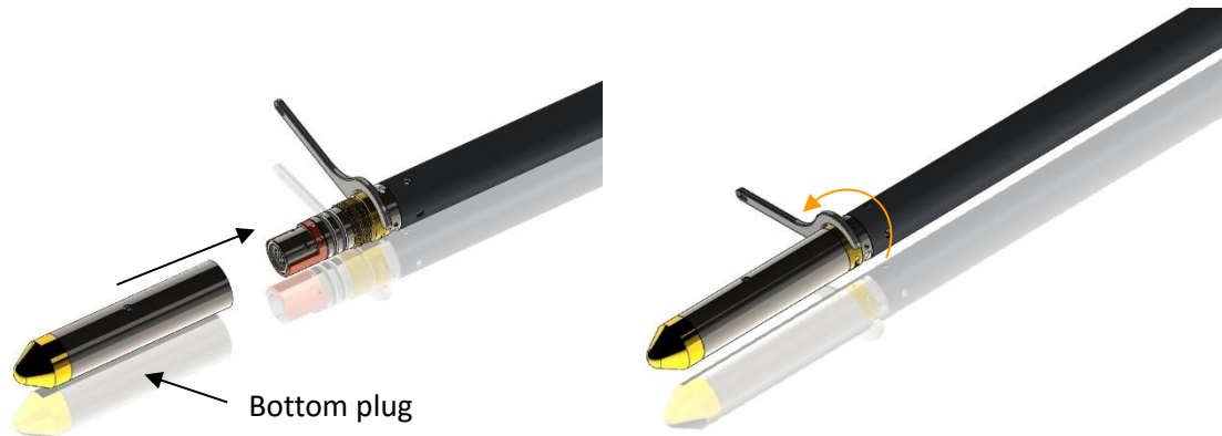
Figure 3-9 Attaching the QL40-Plug
