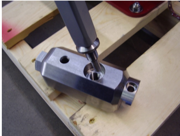
Figure 3-11 Retainer Screw with Source being screwed into Source Carrier
