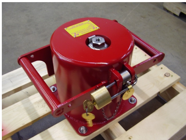
Figure 3-14 Shield with source and source carrier installed
