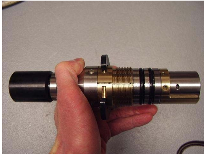
Figure 6-1 Disassembly of the treaded ring
