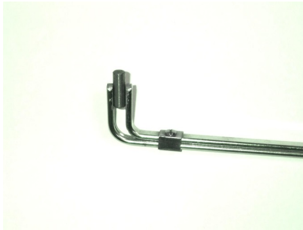
Figure 3-8 Detail of source in tongs
