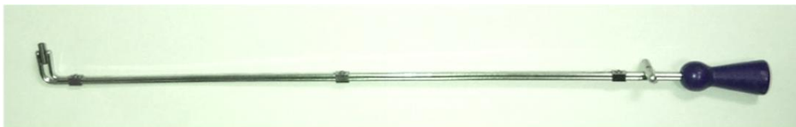
Figure 3-7 Tong with source
