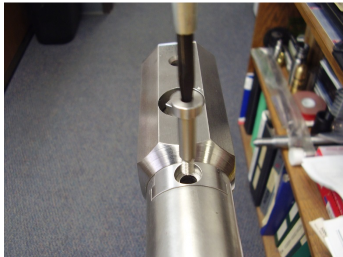
Figure 3-16 Inserting locking screw into the Source Carrier
