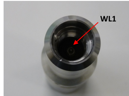
Figure 9-4 MS1 top connection to cable head
