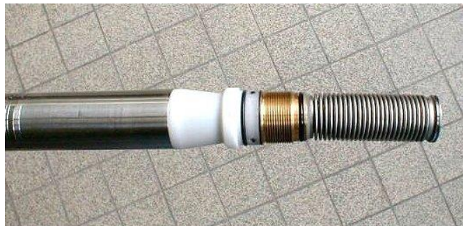
Figure 6-8 Bellows cover removed
