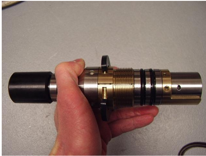
Figure 5-1 Disassembly of the treaded ring
