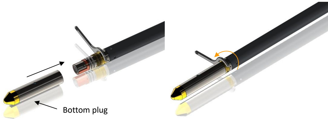
Figure 3-4 Attaching the QL40-Plug
