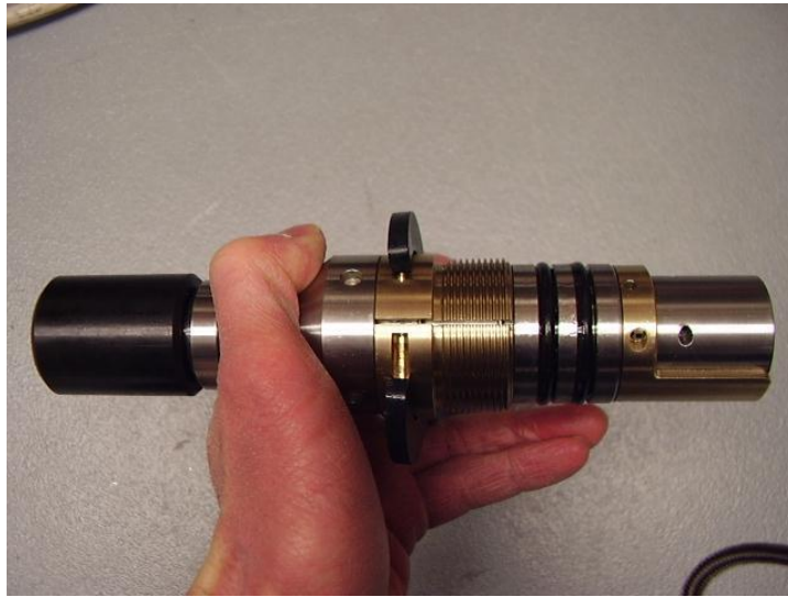
Figure 5-1 Disassembly of the treaded ring
